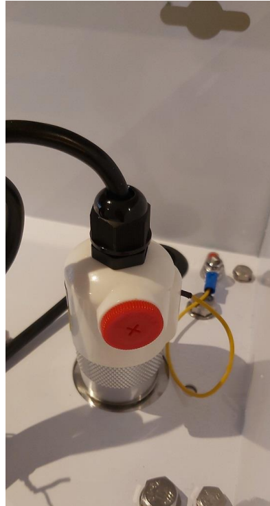
INSERT THE LAMP WITH CAP , AND SLIDE CAP DOWN
