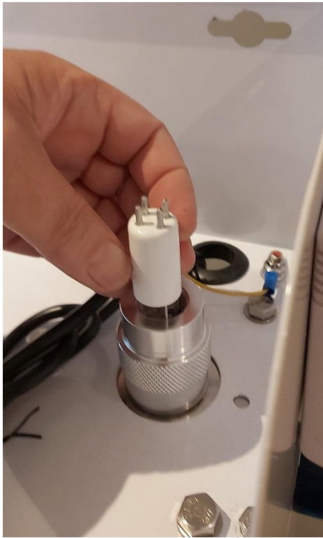
INSERT THE UV LAMP AND HOLD , PLACE 4 PINS CONNECTOR ON LAMP
