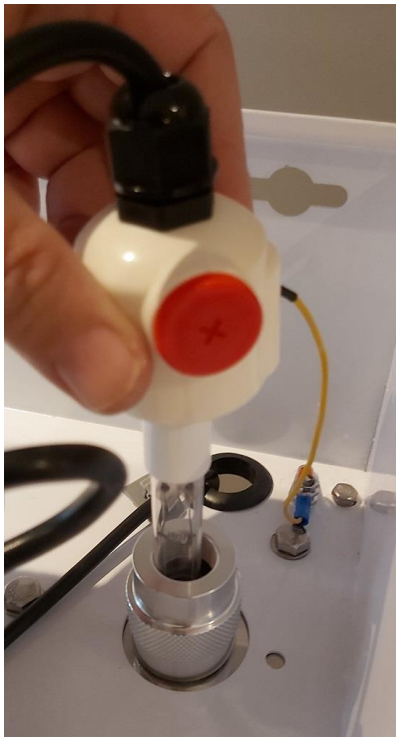
INSERT THE LAMP WITH CAP , AND SLIDE CAP DOWN
